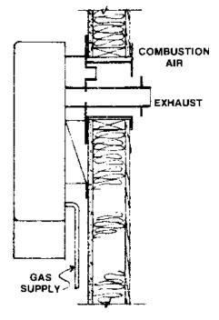
Figure 5: Sealed combusion unit heater.
