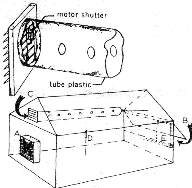
**Figure 1. Components of a ventilated greenhouse.**
