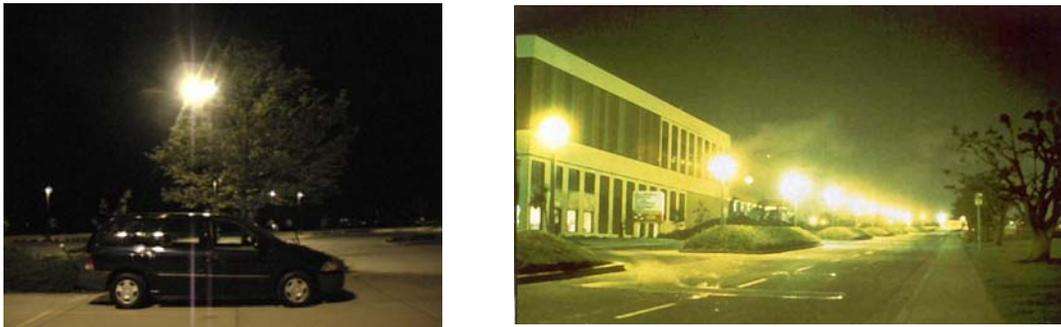
**Figure 2. Examples of direct glare.**
