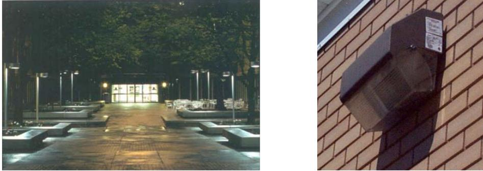
**Figure 4. Fully shielded or IESNA full cutoff luminaires (left) are recommended. Do not use unshielded floodlights or wallpacks (right).**
