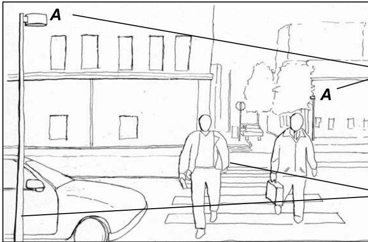
*Full cutoff roadway or pedestrian luminaires provide vertical illuminance on pedestrians and minimize glare to motorists.*
