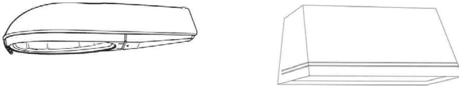
**Figure 7. Examples of IESNA full cutoff luminaires.**
