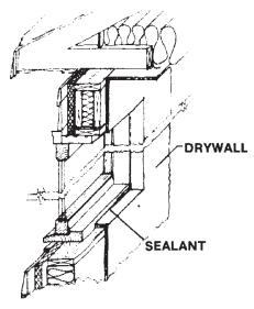
Figure 3: Sealing window openings using the ADA method.
