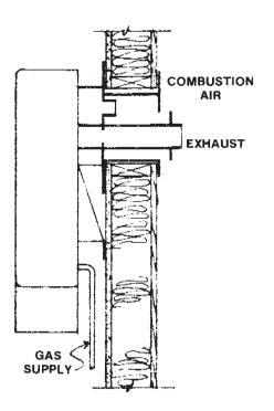
Figure 5: Sealed combustion unit heater.
