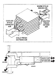
Figure 4: An air-to-air heat exchanger.
