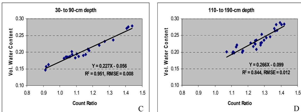
Figure 19. Volumetric soil water content (cm<sup>3</sup>/cm<sup>3</sup>) as a function of the CPN 503DR neutron probe count ratio at the (C) 30- to 90-cm and (D) 110- to 190-cm depths.
