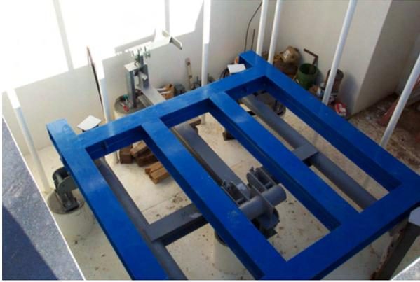
**Figure 5. Steel support frame for the soil tank. This photo also shows the scale.**
