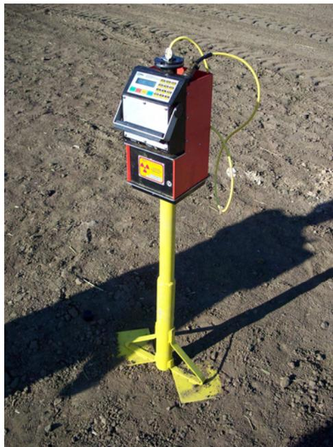
**Figure 14. The neutron probe CPN 503DR sitting on top of the depth-control stand. Photo by Lane Simmons.**
