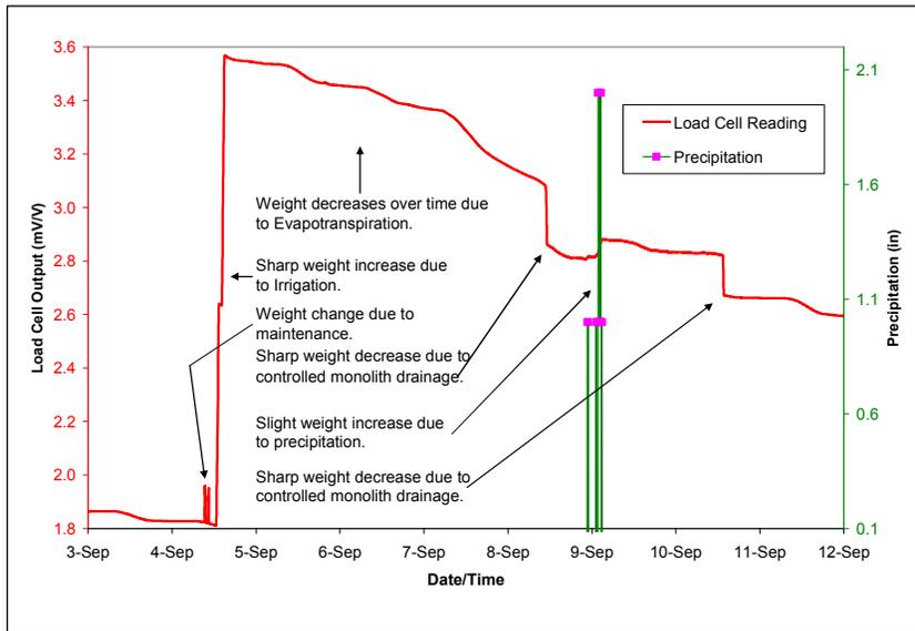
Figure 9. Load cell and precipitation readings for 3-12 Sept. 2006. Graph by Lane Simmons
