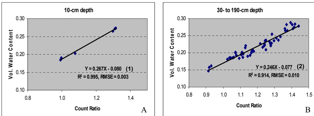
Figure 18. Volumetric soil water content ( $\text{cm}^3/\text{cm}^3$ ) as a function of the CPN 503DR neutron probe count ratio at the (A) 10-cm and (B) 30- to 190-cm depths.
