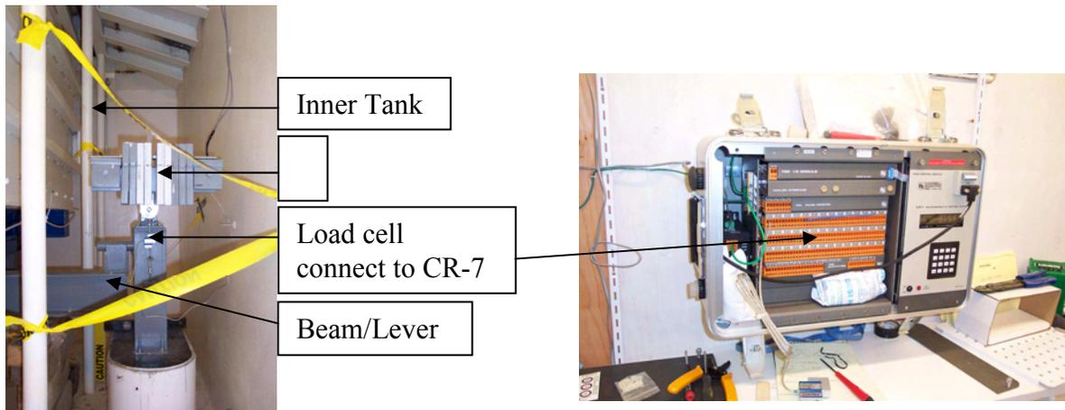
Figure 8. Weighing mechanism and CR-7. Photos by Dale Straw of DWR.
