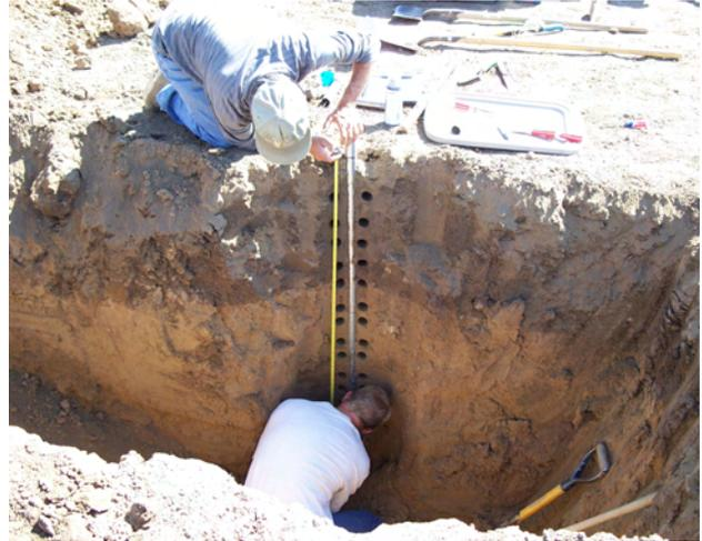
Figure 16. Measuring soil depth before taking soil samples. Photo by Kevin Tanabe.
