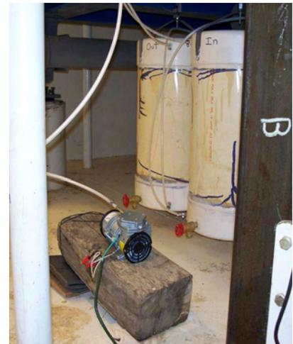
Figure 10. Vacuum pump and drainage tanks. Photo by Dale Straw of DWR.
