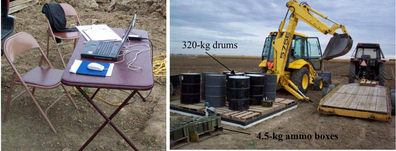
Figure 11. Lysimeter weight calibration.
