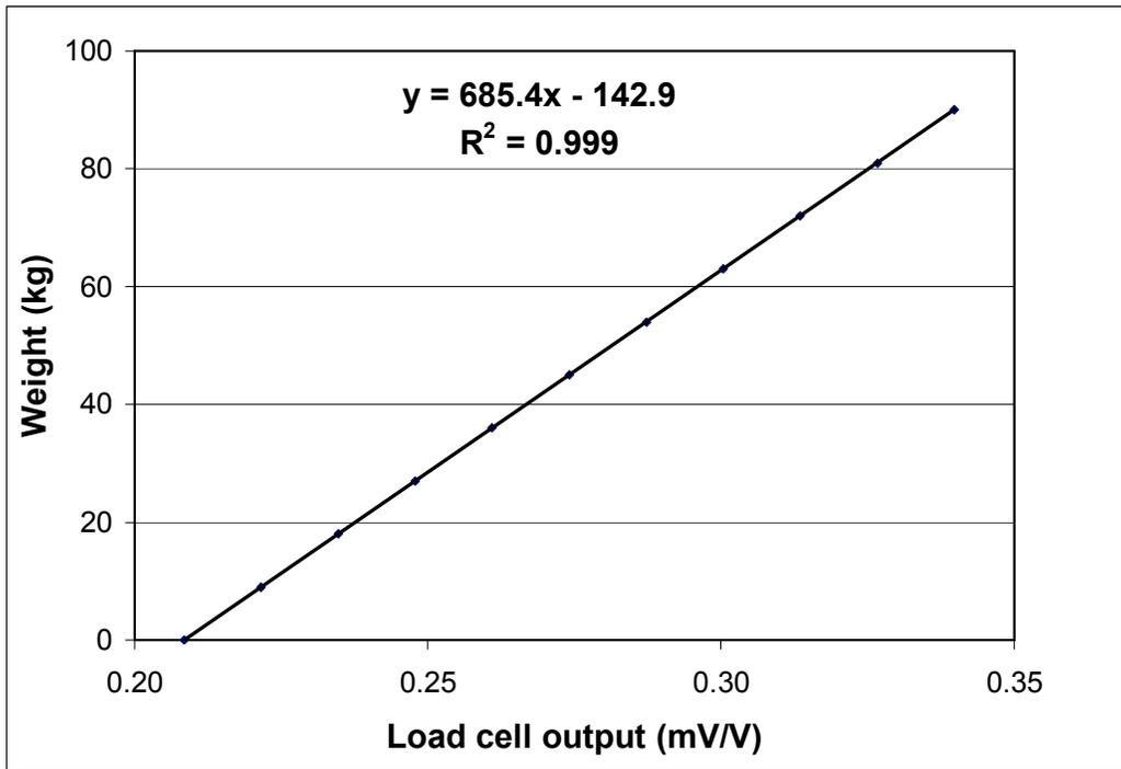
Figure 12. Weight as a function of load cell output. The calibration data was analyzed by Dale Straw of DWR.
