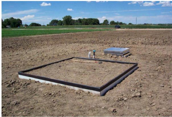
**Figure 7. View of the large lysimeter after the soil around it was repacked.**
