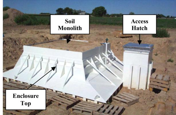
**Figure 6. Enclosure top and access entry to the chamber between the inner and outer tanks.**
