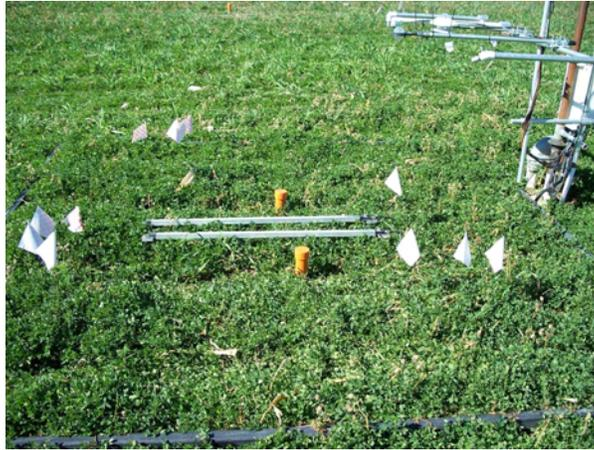
**Figure 13. Neutron probe access tube placement in the soil monolith after it was seeded to alfalfa. The tops of the access tubes are covered with capped PVC pipes painted in orange. The white flags mark the location of various sensors. Two Li-Cor Line Quantum sensors lay between the access tubes.**
