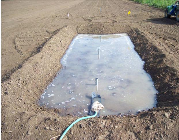
Figure 15. Water being added to the ‘wet’ set of neutron probe access tubes. The ‘dry’ set is in the background. Photo by Lane Simmons.
