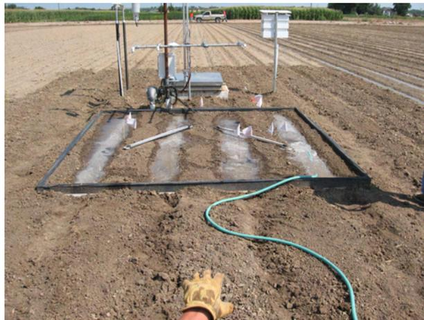
**Figure 21. Water being applied to the soil monolith.
