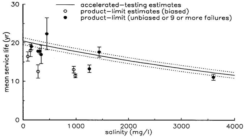
**Figure 11.** Mean service life and its standard error estimated by the generalized accelerated-testing model and product-limit estimates and their standard errors for clothes washers as functions of salinity.
