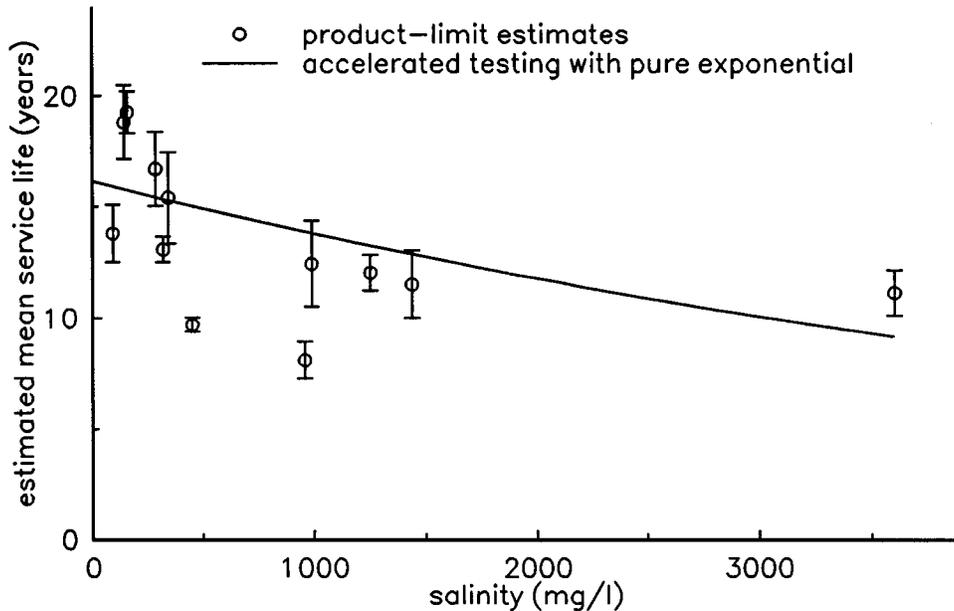
**Figure 4.** Water heater mean life as a function of salinity estimated by a pure-exponential accelerated-testing model and the product-limit method, for which  $\pm$  one standard error is also shown.
