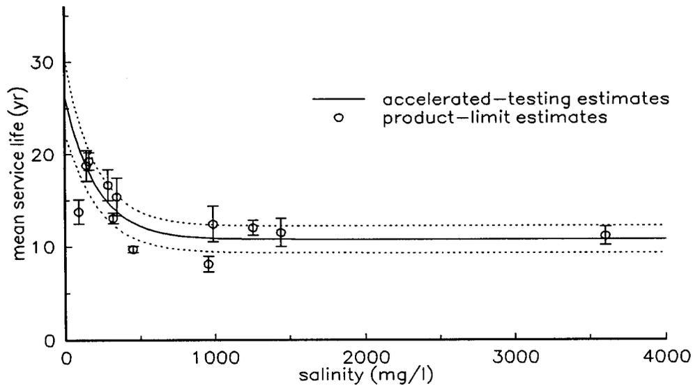
**Figure 10.** Mean service life and its standard error estimated by the generalized accelerated-testing model and product-limit estimates and their standard errors for water heaters as functions of salinity.
